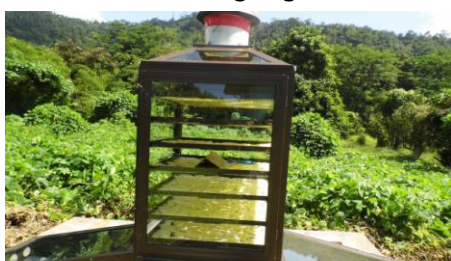
Photo 12: Prototype solar dryer being tested by SROS for drying breadfruit slices for flour production.
