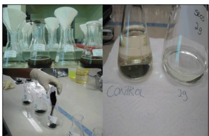
Photo 13: Laboratory experiment on filtration methods to purify coconut oil for cooking purposes.
