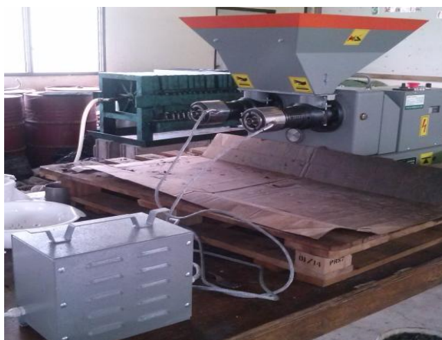
Photo 3: Kent Kraft 40 kg/hour (KK40) oil expeller.
