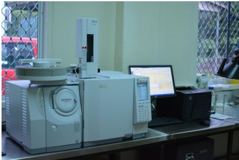
Photo 22: Gas chromatography/mass spectrometry analytical equipment which is used for analysis of methamphetamine and its precursors.
