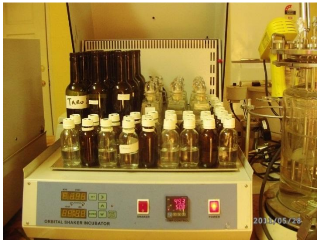
Photo 6: Accelerated testing procedure using an incubator.
