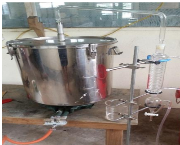
Photo 11: 65-L pot still for essential oil extraction.
